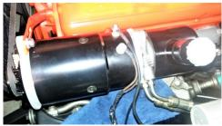
**9029** install all hoses at pump and at valve. Use line wrenches to tighten connections. FILL PUMP WITH FLUID! USE
