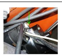
Install large end of charge wire to battery terminal post on starter solenoid, or charge wire can be connected to the positive post of the battery.
