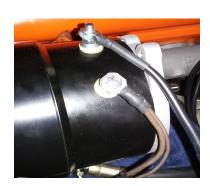
Install small end of new black charge wire to the terminal tagged "B+". Route charge wire to starter solenoid. **9029V** For installation with ammeter see special instructions.
