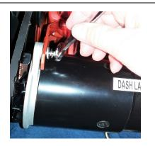
Install belt and adjusting brace with hardware provided. Tighten brace, tension belt as per shop manual.
