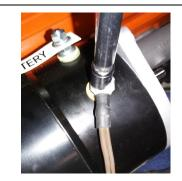
**9029, 9005,** for correct Dash Lamp operation, attach your existing double brown wire to the unlabeled alternator terminal (see pic). Insulate ends of remaining generator wires and tuck them into existing harness. **9029V** this terminal can be left bare or a dummy wire can be installed for appearances.
