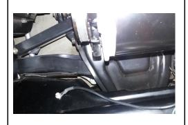
Install other end of ground wire to engine, frame, or front sheet metal. Be sure all OEM ground straps are installed on vehicle.
