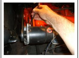
Remove adjusting brace hardware and remove belt. Remove lower mounting hardware and remove generator. Check bracket size in next step.
