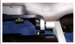
Install one washer between the rear frame and the bracket to achieve a good fit. Snug the hardware just enough to still allow the alternator to pivot. Do not overtighten.
