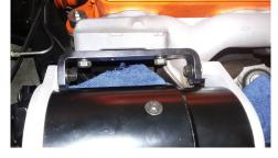
Install new alternator onto bracket using hardware provided. Install washers under the bolt heads and under the nuts. SEE NEXT STEP TOO -----»
