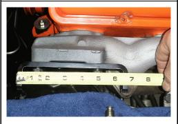
Verify the existing bracket length, measured from outside to outside of the mounting ears, use this chart to determine the correct length you need:
