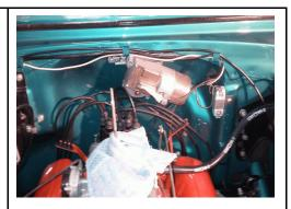
**9029, 9005,** charge wire can be routed along with existing firewall wiring harness or radiator core support harness.
